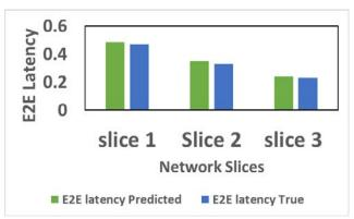
Fig. 2 Predicted E2E Latency vs True Latency
